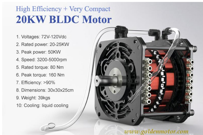
Figure 5. BLDC electric motor. Source: Goldenmotor.com
