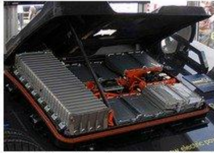
Lithium ion battery pack.
