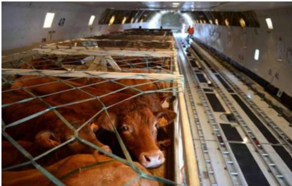
Slika 21. Prijevoz krava teretnim zrakoplovom u otvorenom kontejneru, Izvor: <https://hr.blabto.com/2606-transportation-of-livestock-methods-requirements-doc.html>
