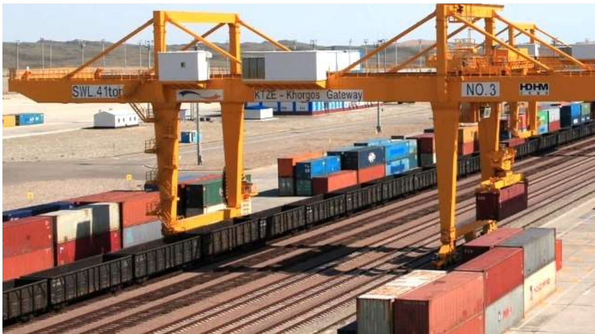
Slika 10. Terminal za utovar kontejnera na vagonе, Izvor: https://www.maritime-executive.com/editorials/can-the-new-silk-road-compete-with-the-maritime-silk-road
