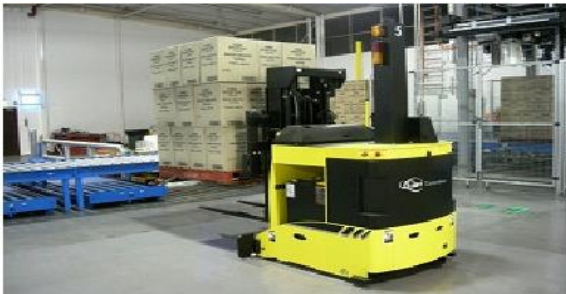
Slika 31. Automatski vođeni viličar, Izvor: https://www.researchgate.net/profile/Marcelo-Becker/publication/224141565/figure/fig1/AS:302651041435648@1449169039118/AGV-Automated-Guided-Vehicle-working-in-an-Intelligent-Warehouse-in-Germany-2.png
