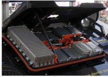
Lithium ion battery pack.
