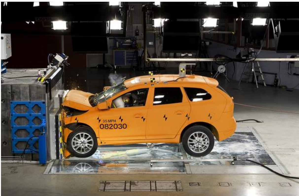
Figure 9. Car crash testing
