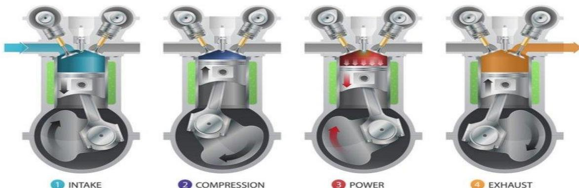
Slika 16. Princip rada četverotaktnog Otto motora, Izvor: [https://www.researchgate.net/figure/Four-stroke-cycle-engine-20\\_fig1\\_334568325](https://www.researchgate.net/figure/Four-stroke-cycle-engine-20_fig1_334568325)
