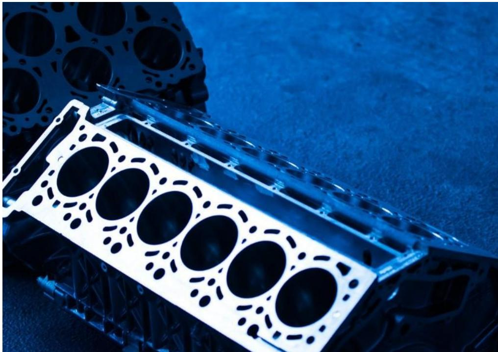
Slika 8. Blok motora, Izvor: <https://www.motor.com.hr/blok-motora-je-temelj-automobila/>
