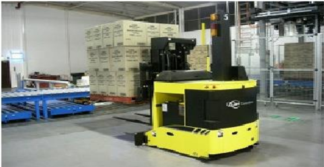
Slika 31. Automatski vođeni viličar, Izvor: https://www.researchgate.net/profile/Marcelo-Becker/publication/224141565/figure/fig1/AS:302651041435648@1449169039118/AGV-Automated-Guided-Vehicle-working-in-an-Intelligent-Warehouse-in-Germany-2.png
