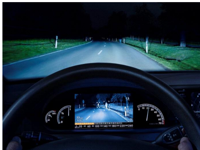
Figure 5. Combination of active and passive night vision
